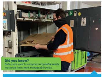
The waste is separated into cardboard, clear plastic and coloured plastic at NVS' warehouse. Once separated, the waste is fed into our baler machines ready to be collected by our recycling partner.
